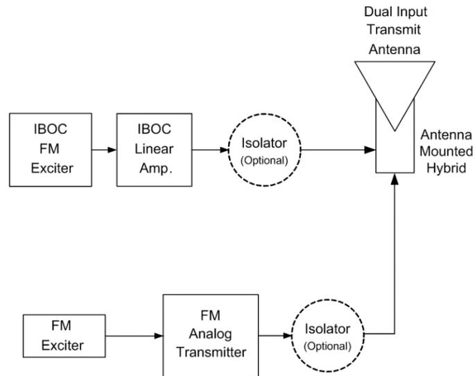
**Figure 5: FM HD Radio Dual-Input Antenna Implementation**
