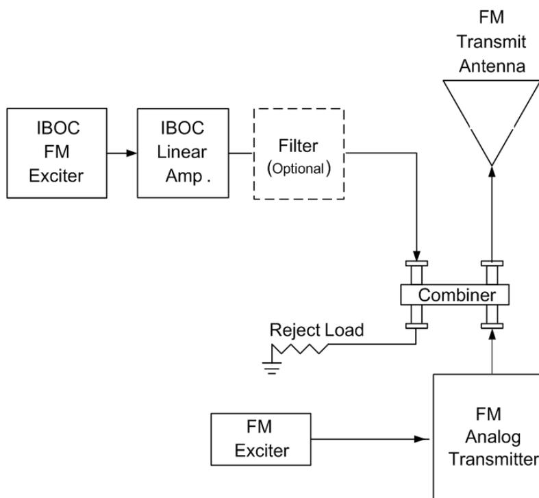
**Figure 2: FM HD Radio high-level, separate amplification**
