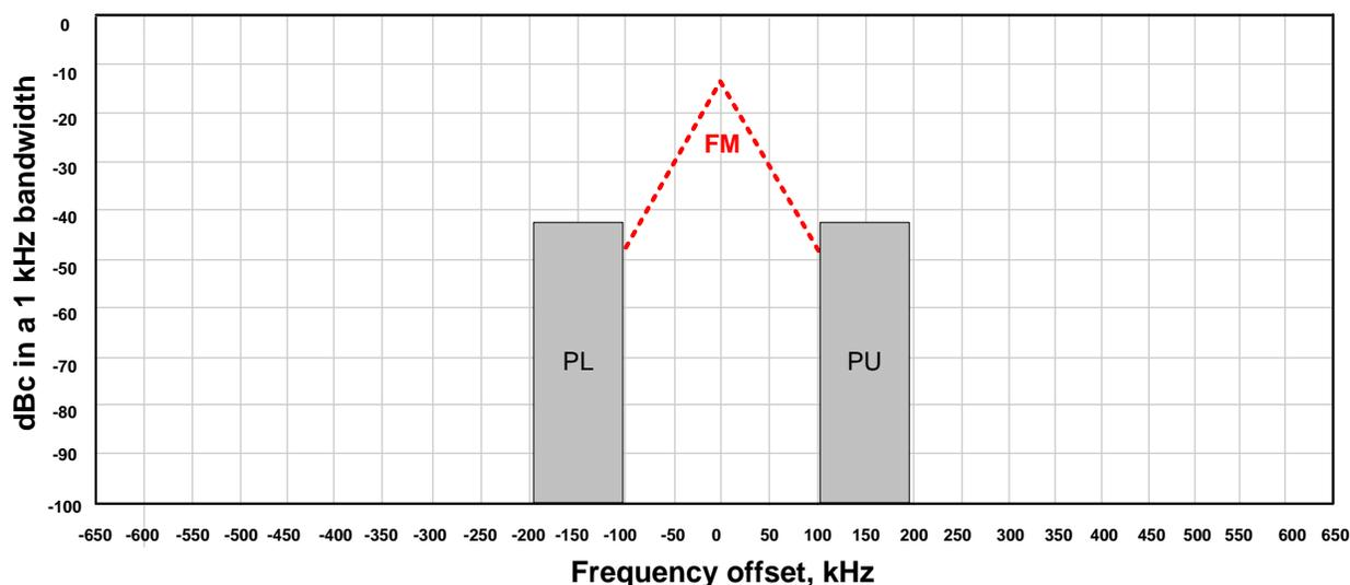
**Figure 1: Hybrid analog FM and HD Radio signals**
