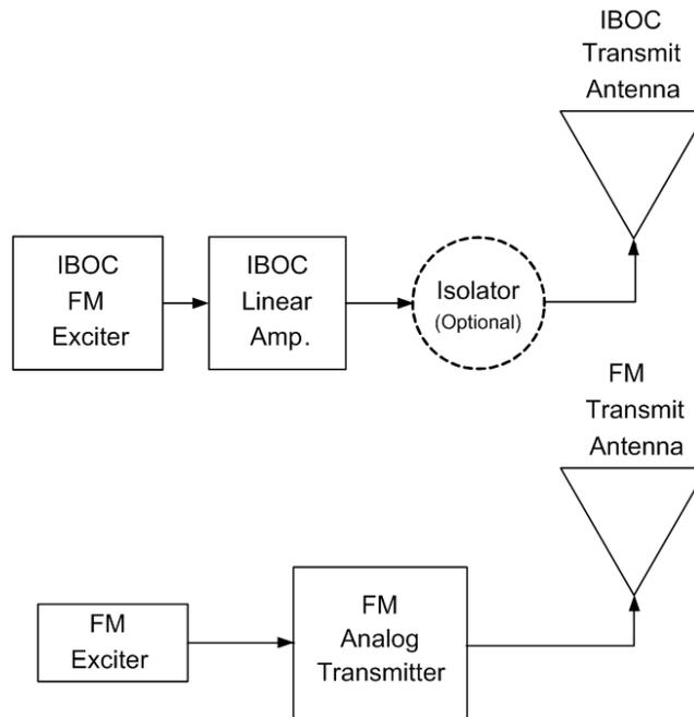
**Figure 4: FM HD Radio Separate Antenna Implementation**
