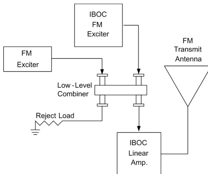
**Figure 3: FM HD Radio low-level, common amplification**
